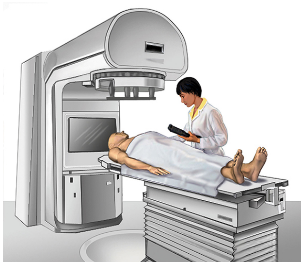
Figure 1. Linear accelerator for external beam radiation therapy (from www.cancer.gov )
