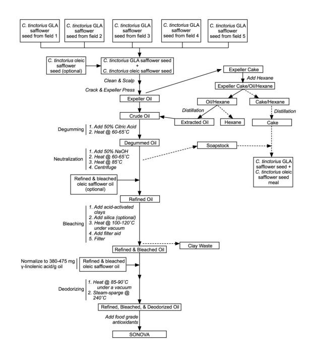
Figure 2. Production Process for SONOVA
