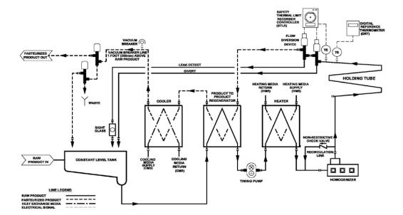
Figure 32. HTST Pasteurizer with a Homogenizer Located at the Outlet of the Heater Section and of a Larger Capacity than the Timing Pump
