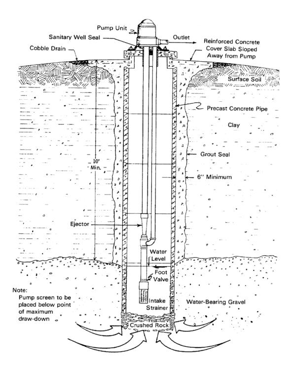
Figure 15. Dug Well with Two-Pipe Jet Pump Installation
