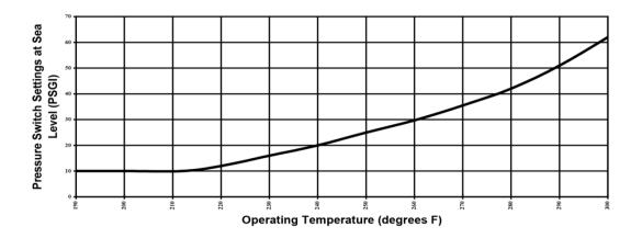
Figure 57. Pressure Switch Setting
