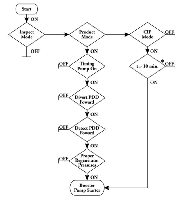
Figure 56. Logic Diagram: HTST Booster Pump
