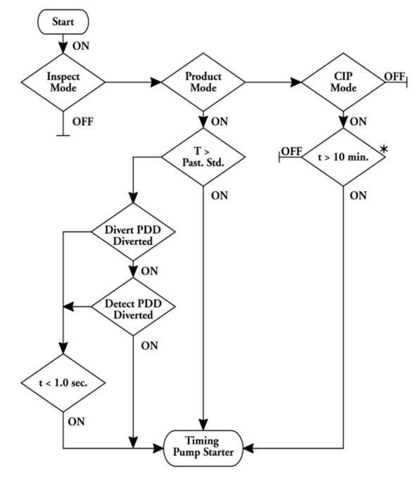
Figure 55. Logic Diagram: HTST Timing Pump
