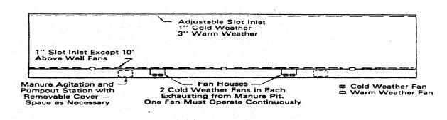
Figure 6. Schematic Diagram Showing Suggested Exhaust Fan Locations for a Typical Stall Dairy Barn with Gutter Grates Over Liquid Manure Storage
