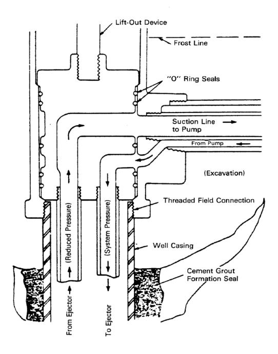
Figure 24. Pit-less Unit with Concentric External Piping for Jet Pump Installation
