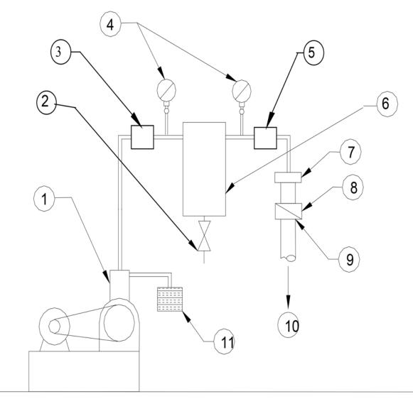
Figure 44. Individual Compression-Type Air Supply
