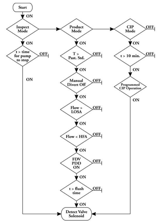
Figure 53. Logic Diagram: HTST Flow-Diversion, Leak-Detect Valve Stem
