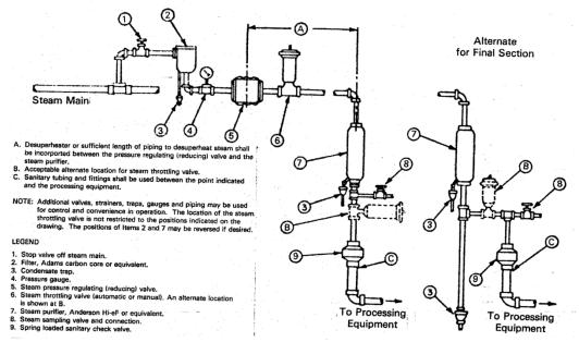
Figure 50. Culinary Steam Piping Assembly for Steam Infusion or Injection (Optional Configuration)
