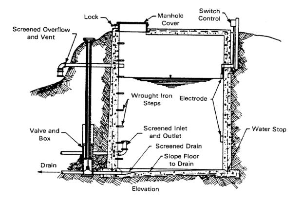
Figure 21. Typical Concrete Reservoir
