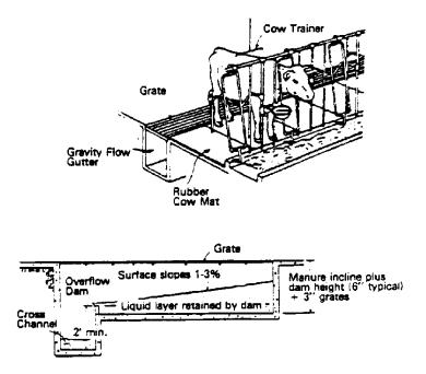
Figure 1. Side Cross Section of a Gravity Flow Gutter
