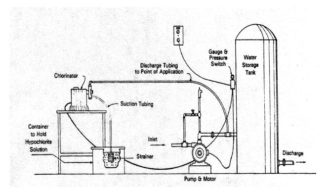
Figure 30. Positive Displacement Chlorinator
