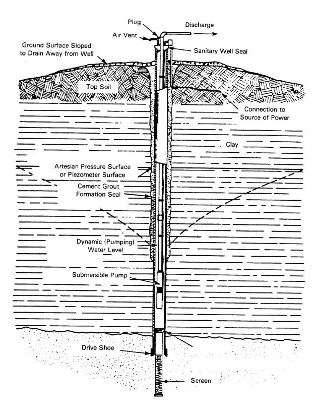
Figure 14. Drilled Well with Submersible Pump
