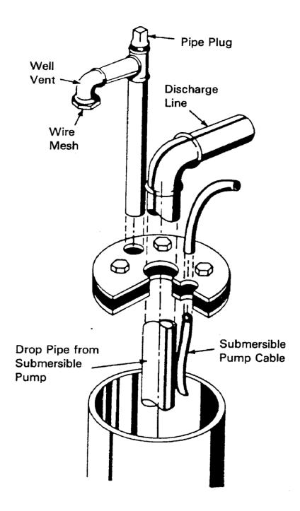
Figure 27. Well Seal for Submersible Pump Installation
