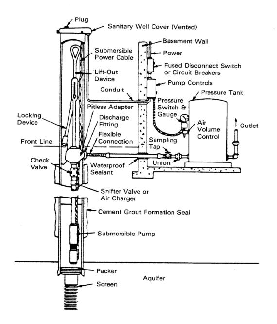
Figure 22. Pit-less Adapter with Submersible Pump Installation for Basement Storage
