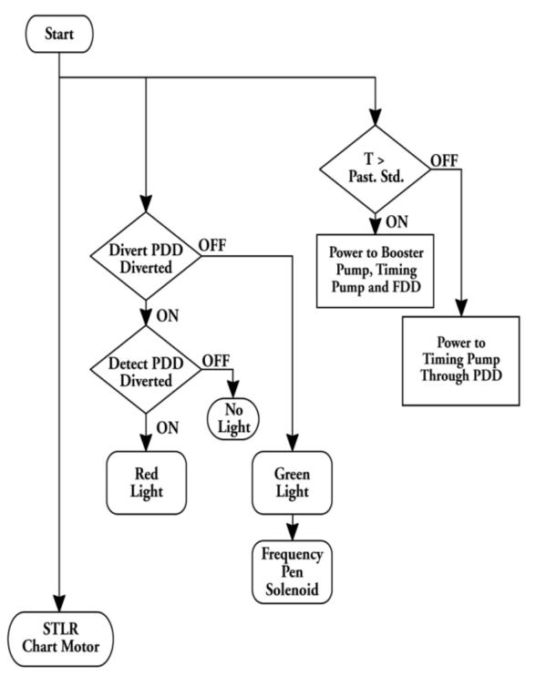
Figure 54. Logic Diagram: HTST Safety Thermal Limit Recorder-Controller
