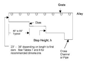
Figure 2. Stepped Gravity Flow Gutter
