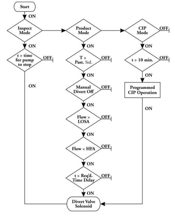
Figure 52. Logic Diagram: HTST Flow-Diversion Device, Divert Valve Stem
