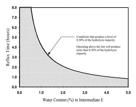
The area below the line in the plot above could be proposed as the design space.
