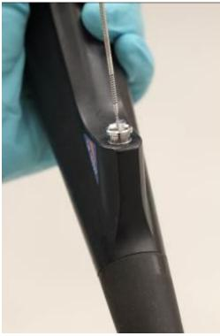
A5.3.5.6 Instrument channel brush exiting distal end
