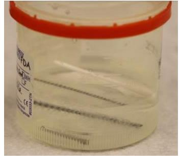
Sample container with liquid extract and swab and brush heads (prior to A5.3.6)
