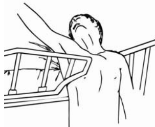
Zone 7 – Entrapment between head or foot board and the mattress end
