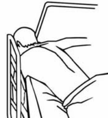
Zone 6 – Entrapment between the end of the rail and the side edge of the head or foot board
