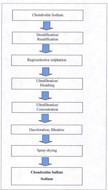
Figure II.G.2. Production of Chondroitin Sulfate Sodium (Chemical Synthesis)
