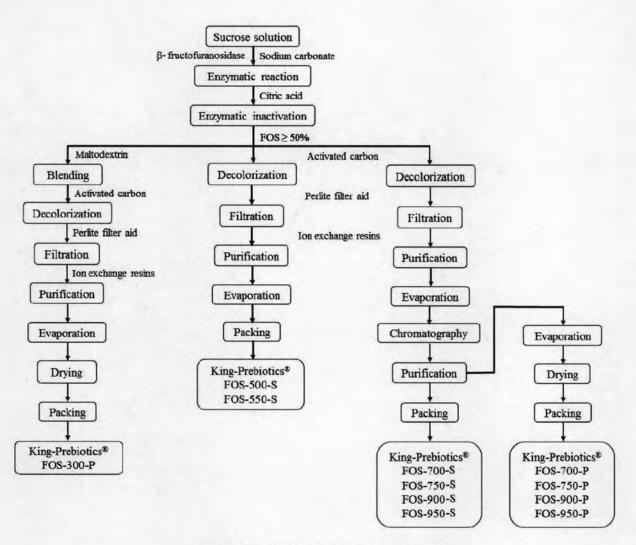
Figure II.G.1. Manufacturing Process of FOS
