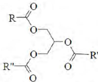
Where R, R' and R'' = an epoxidized hydrocarbon chain
