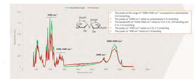
Figure 2.2.3-1 A Comparison of the Spectra from DouxMatok Sugar with Sucrose<sup>a</sup>
