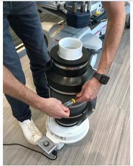
5. Slide the loosened hose clamp down. Remove top black filter case.
