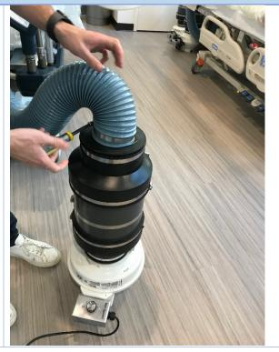
4. Remove screw from the hose clamp connecting the black top filter case to the main grey filter case using a screwdriver.
