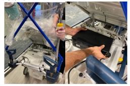
Regular Floor/ICU Beds: 13. Plug the HVAC system into any of the "Battery Backup" outlets of the battery supply box. 14. Plug the battery backup box into an external outlet. 15. Turn the fan on by setting the dial at the bottom of the fan to HIGH. 16. Test the system by letting the fan run for a few minutes and visually inspect the tent for hour-glass shape. (This is the indication for negative pressure.) a. Additionally, check negative pressure indicator
