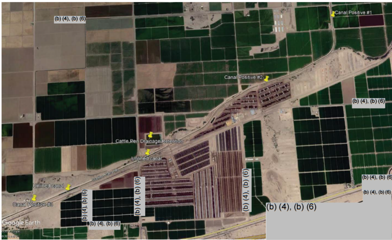
Figure 1. Wellton Irrigation Canal. This Google Earth view depicts a section of the Wellton main canal adjacent to a CAFO and locations of three outbreak-pathogen-positive irrigation water samples. The sample locations are upstream, adjacent to, and downstream of the Wellton-area CAFO. Also noted are unlined irrigation canal sections and a CAFO retention pond. Water in the canal flows from west (left) to east (right) in the figure above. The CAFO at the bottom center of Figure 1. See Figure 2 for an enlarged image of the CAFO.
