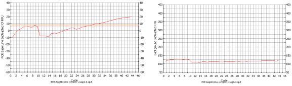
Figure 5: Amplification plot of a sample with a "wandering" curve (left) and the corresponding background fluorescence view (right).
