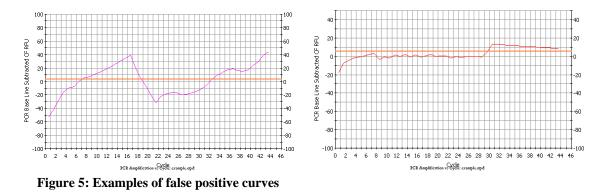
• To better understand and evaluate challenging curves more effectively, use the background fluorescence view (Rn versus Cycle with AB software) to determine if the curve is actually positive. In this view, a sharp increase in fluorescence indicates a true positive while a flat line (or wandering line) indicates no amplification.
