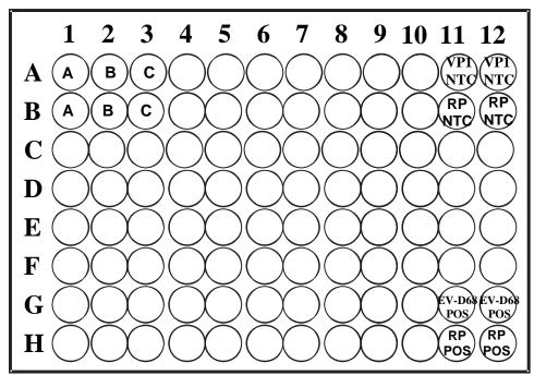
RNase positive control (RP POS); No template reaction mix controls (NTC); EV-D68 2014 positive control (EV-D68 POS); A, B and C (samples)
