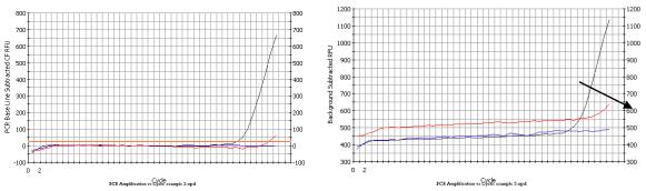
Figure 7: Amplification plot of three samples in the linear view (left) and the corresponding background fluorescence view (right)
