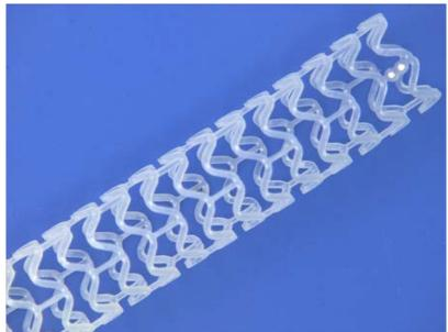
Figure 2-2. Digital Photograph of the 3.5 mm Medium BVS in Expanded Form
